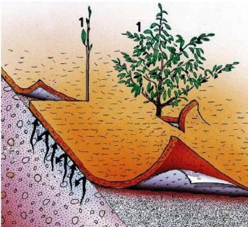
All joints should be overlapped by 150mm to ensure no daylight penetration. Pin the
