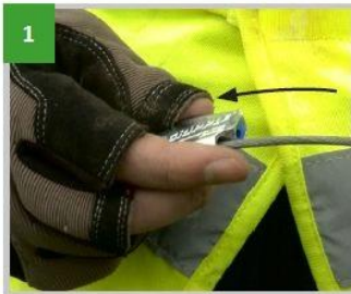
1 Thread guy wire through the tensioner
