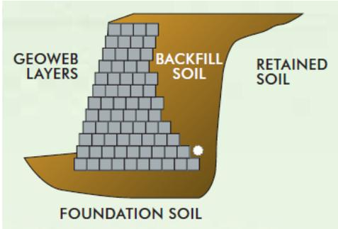
The perforations in Geoweb allow lateral drainage through the system, In vegetated systems, the perforations increase root lock-up, creating a more stable vegetated mass and overall healthier soil environment. The Geoweb panels can be stepped back to create the wall inclination required based on space available and planting requirements
